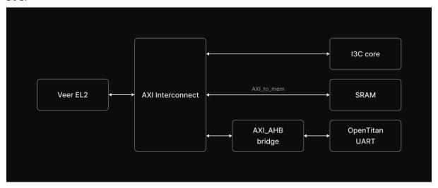
The Guineveer reference System-on-Chip (SoC) design employs the VeeR EL2 core which is a 32-bit CPU supporting RISC-V's extensions for integer (I), compressed instruction (C), multiplication and division (M), and instruction-fetch fence, CSR, and subset of bit manipulation instructions (Z).
